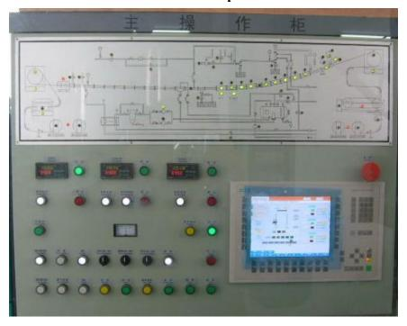
Set total line flow diagram, LED display, clear.
